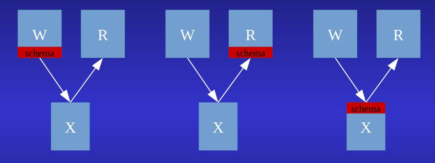
schema on write (enforce valid data) schema on read (NoSQL) schema with data (SQL, OO)
