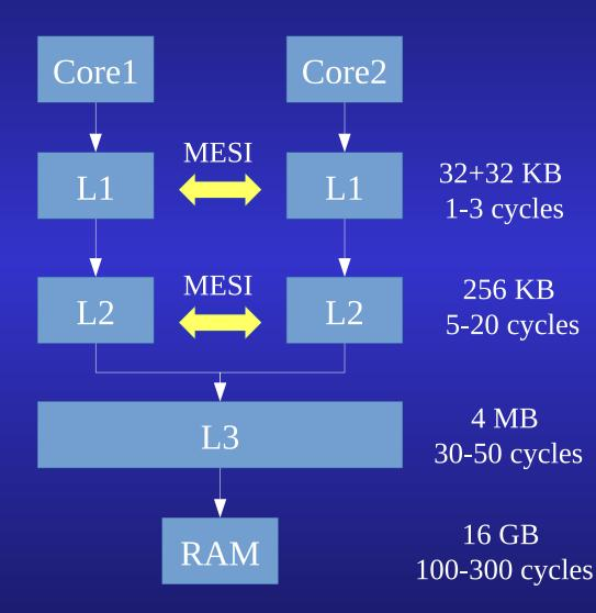
Caches have to communicate to ensure coherent view
