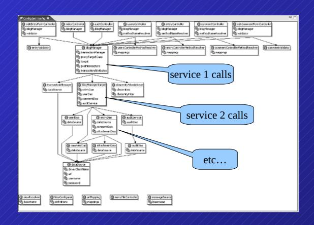
Example of Spring dependency graph showing inter-component (i.e. service) connections
