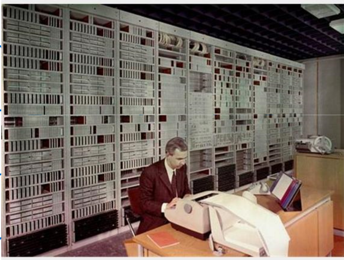
Ericsson's AKE12 Switch 1968 - Computerized Electromagnetic code switching
